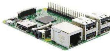
**Figura 10. Raspberry Pi 3 modelo B**
